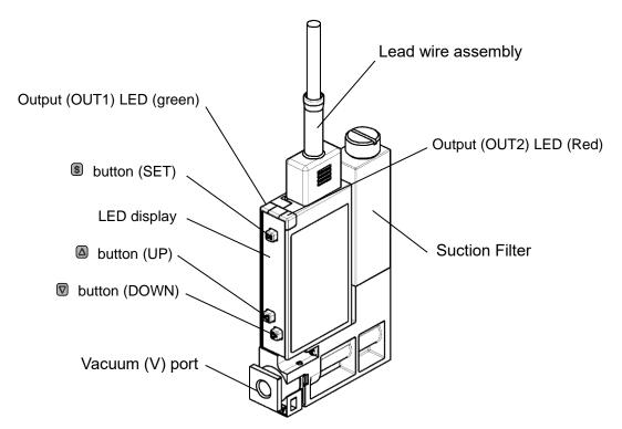
Output (OUT1) LED (green): LED is ON when the switch output (OUT1) is ON.
