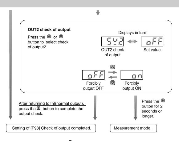
\* : Return to measurement mode from any point by pressing the S button for 2 seconds or longer.
