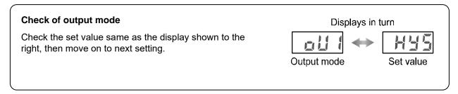
Press the 🖲 button to set. 🔻 Move on to setting of reversed output.
