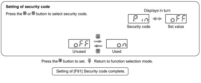
If the security code is used, it becomes necessary to enter the security code to release the key lock. The security code number can be set to a different value by an operator. The default setting is "000".
