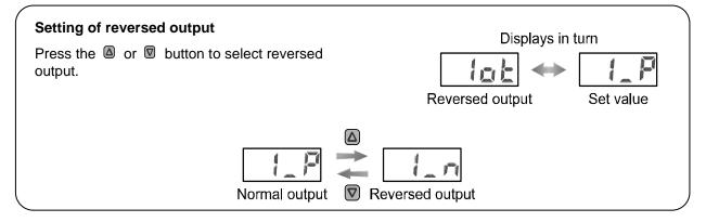
Press the  $\$  button to set.  $\$  Move on to setting of pressure.
