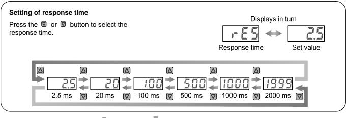
Press the S button to set.  $\P$  Return to function selection mode.
