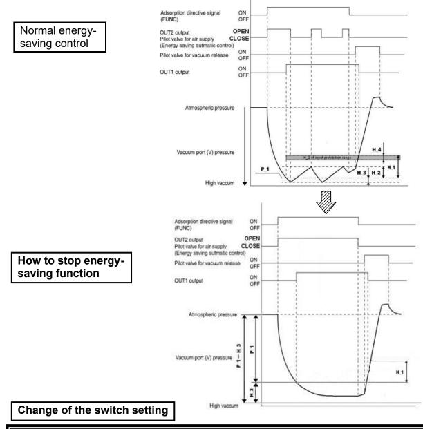
For stopping the energy-saving function, change the setting of H\_3 to P\_1 – H\_3  $\leq$  -100. Refer to page 25 [F 2] OUT2 setting for the setting of H\_3.
