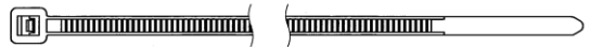
Tie band 1 pc. Used for tying and fixing the \Phi 4 tube and switch cable. \Phi 4 tube is connected to release pressure supply port (PD) when release pressure is supplied to this product.
