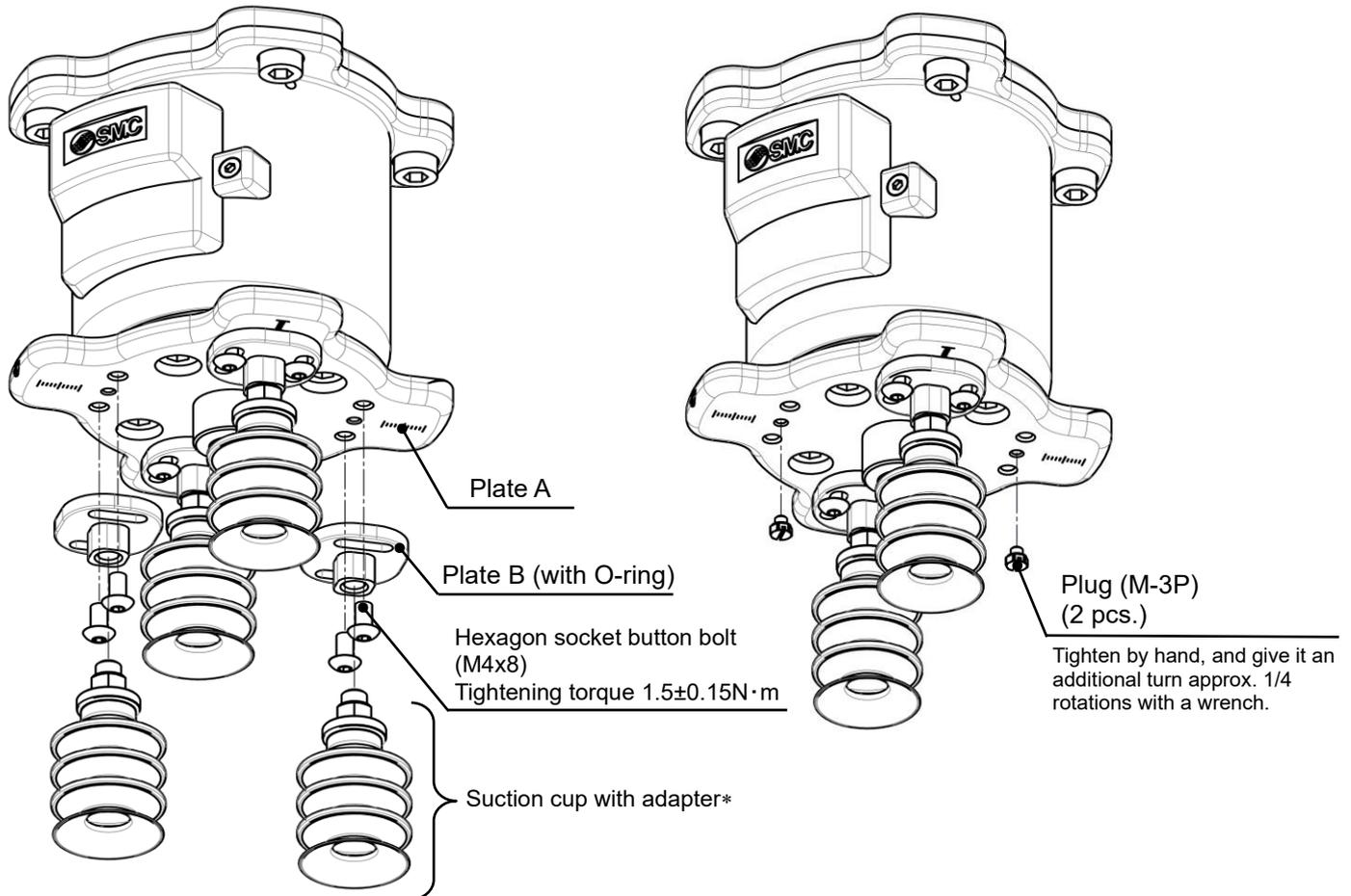
(1) Disassemble the suction cups with adapter
