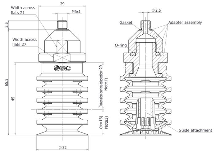
Note1) "D" and (st) indicate the reference value during gripping at vacuum pressure: -85[kPa].
