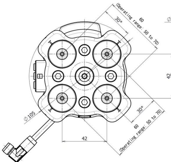
\*Operating range: 25 to 35 (When a cup is mounted in the center)
