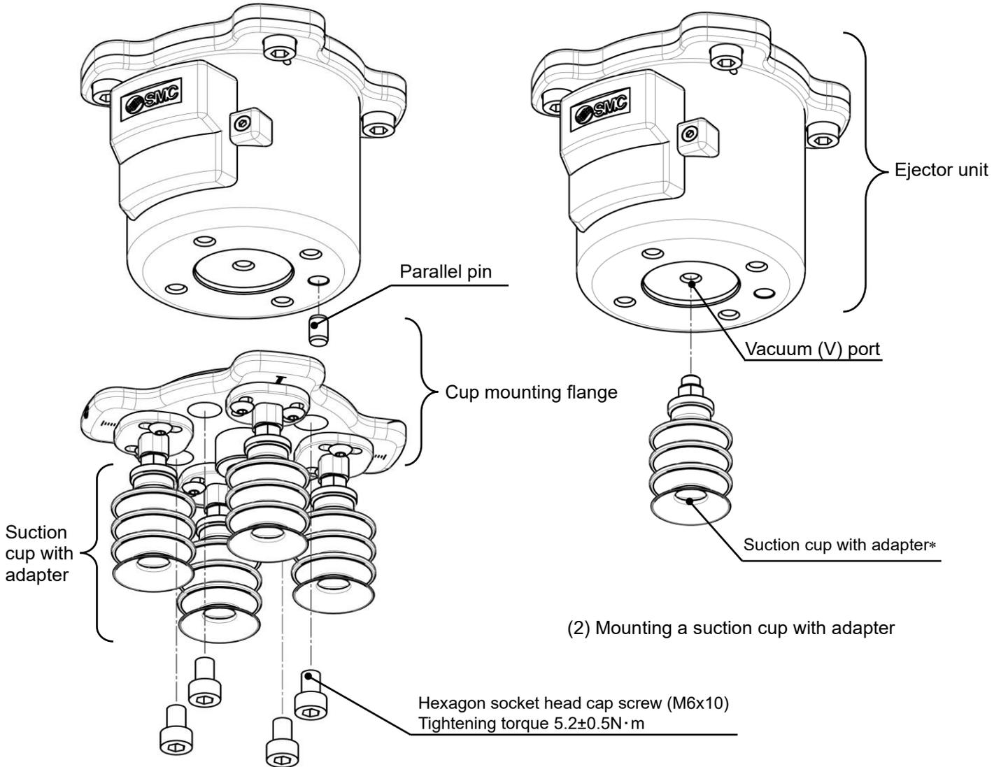
(1) Disassemble the cup mounting flange
