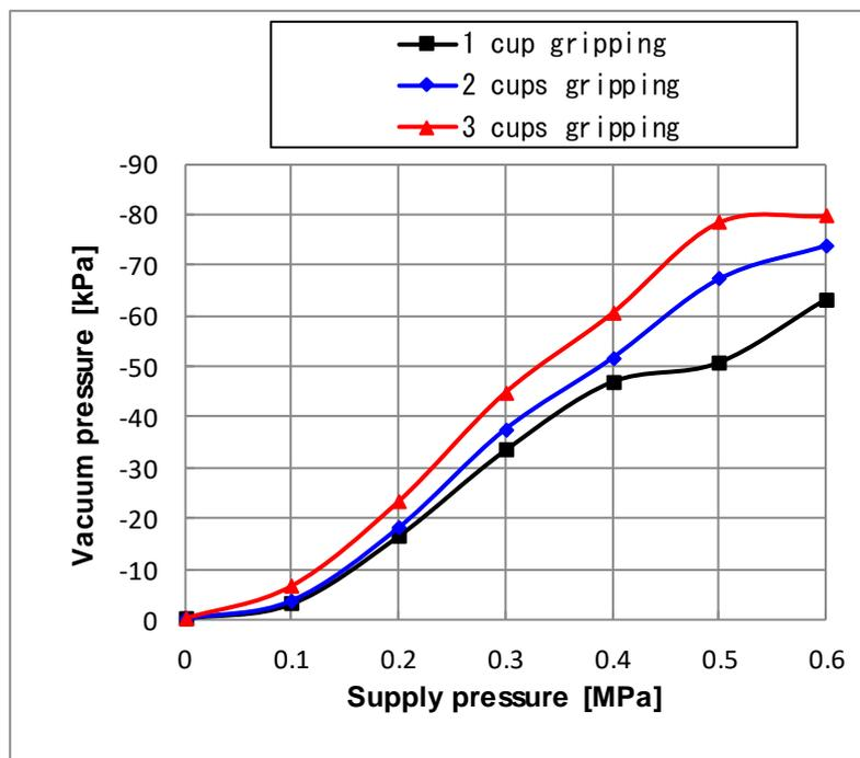
Exhaust Characteristics by using the vacuum saving valves: ZP2V-B06-05
