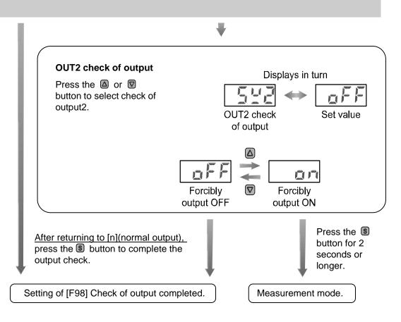
\*: Return to measurement mode from any point by pressing the
