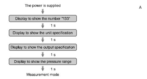
See below for the energy saving control operation and the set values which are preset to the switch.
