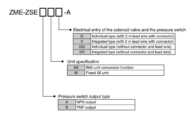
Integrated cable assembly for the solenoid valve/pressure switch
