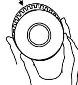
Fig. 2 Removal of the piston seal
