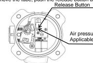
Air pressure supply (P) port Applicable tubing O.D.: Ф4
