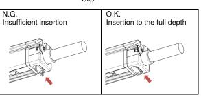
(3) Install the bar and insert the branch cable into the controller and fix it with screw
