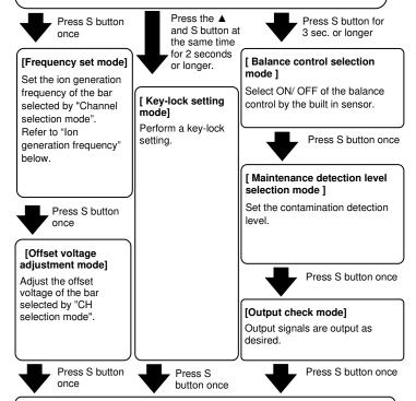
Note) In each setting mode, the selected bar moves on to the ion generation stop mode by pressing  $\nabla$  and  $\triangle$  button simultaneously for 2 s or longer and stops the ion generation (Operation is not possible while the key lock is ON or externally input signal is ON). To release, press the S button once or turn the power off and on
