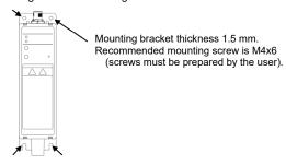
· Use an optional DIN rail mounting bracket. After installing the DIN rail mounting bracket, fix the bracket to the DIN rail
