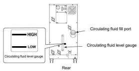
If the circulating fluid is supplied over the specified level, follow the procedure provided in the operation manual section 7.3.1 "Draining of circulating fluid out of tank" to drain excess fluid until it reaches the specified level.
