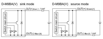
The number shown in brackets [] in the wiring diagram indicates the pin number of a pre-wired connector.
