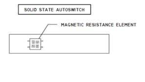
AS THE MAGENT IS BROUGHT CLOSER, THE SENSOR RESISTANCE CHANGES WHICH CAUSES THE ELECTRICAL POTENTIAL TO FLUCTUATE WHICH IS IDENTIFIED BY THE IC, CREATING OUTPUT.
