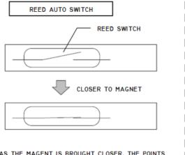
AS THE MAGENT IS BROUGHT CLOSER, THE POINTS WHICH WERE SEPARATED BEGIN TO MOVE AND AN ELECTRIC CURRENT IS GENERATED WHEN THESE COME INTO CONTACT.
