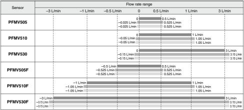
The values shown on the graph are the displayed flow rate range and set flow rate range when PFMV5 series and PFMV3 series are connected.
