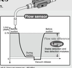
(Comparison under Nozzle diameter: ø0.3, Vacuum pressure: -60 kPa)
