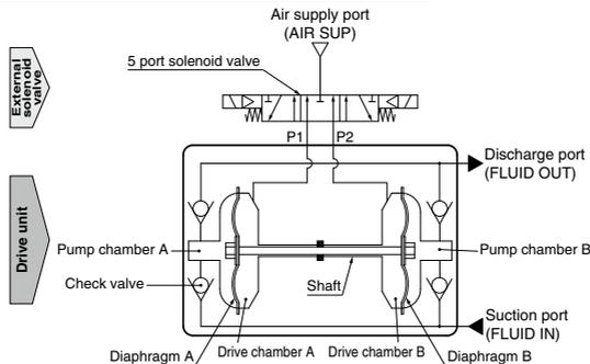
1. When air is supplied to P1 port, it enters drive chamber A.
