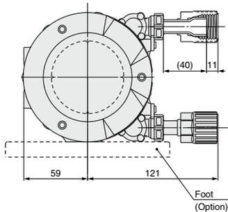
**Dimensions: Automatically Operated Type (PAF5000 Series)**
