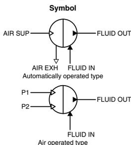
Note 1) The port size of the pilot port is as follows. Automatically operated type is 1/4"; Air operated type is 1/8".
