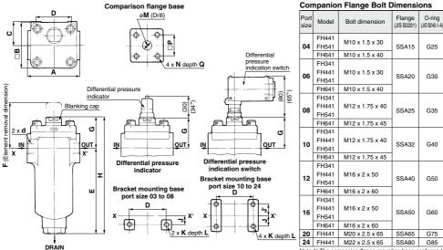
Note 1) The companion flange mounting base conforms to JIS B 2291 (21 MPa pipe flanges for hydraulic use) SSA.
