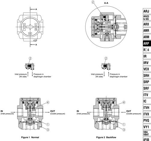
When the inlet pressure is higher than the set pressure, the check valve (2) closes and operates as a normal regulator (Figure 1). When the inlet pressure is shut off and released, the check valve (2) opens and the pressure in the diaphragm chamber (1) is released to the inlet side (Figure 2).
