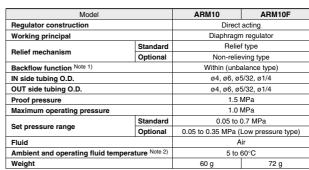
Note 1) 0.1 MPa or greater set pressure is required when used in the reverse flow. Note 2) 5 to 50°C when the digital pressure switch will be used.
