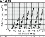
Note) The graph above shows the relief flow when the set pressure rises and falls from 0.1 MPa
