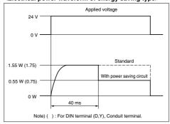
Since the voltage will drop by approx. 0.5 V due to the transistor, pay attention to the allowable voltage fluctuation. (For details, refer to the solenoid specifications of each type of valve.)
