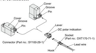
\* In order not to damage the connector and cover, do not pull the lead wire excessively (with a force of 30 N or more).
