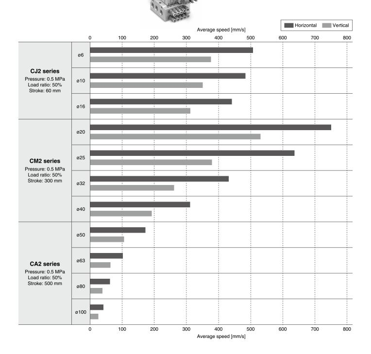
Cylinder for horizontal use are based on the coefficient of rolling friction 0.1.
