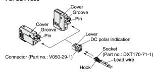
In order not to damage the connector and cover, do not pull the lead wire excessively (with a force of 10 N or more).
