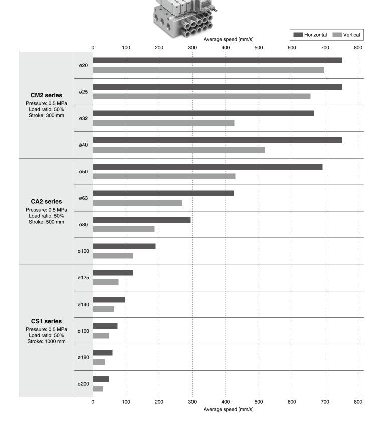
Values at extension of a directly coupled cylinder when meter-out speed controllers are used with the needle full open.
