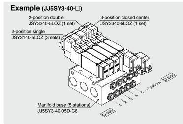
JJ5SY3-40-05D-C6-1 set (Type 40 5-station manifold base part
