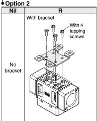
Options are shipped together with the product but do not come assembled. When only optional parts are required, refer to Option 2/Part Nos. below.
