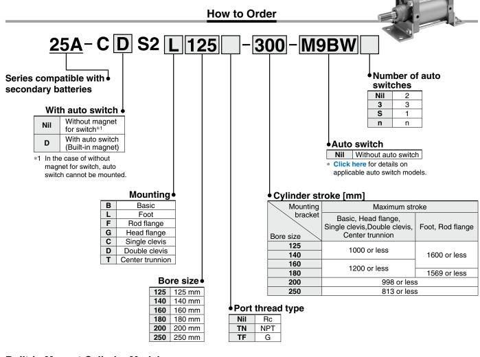
Built-in Magnet Cylinder Model
