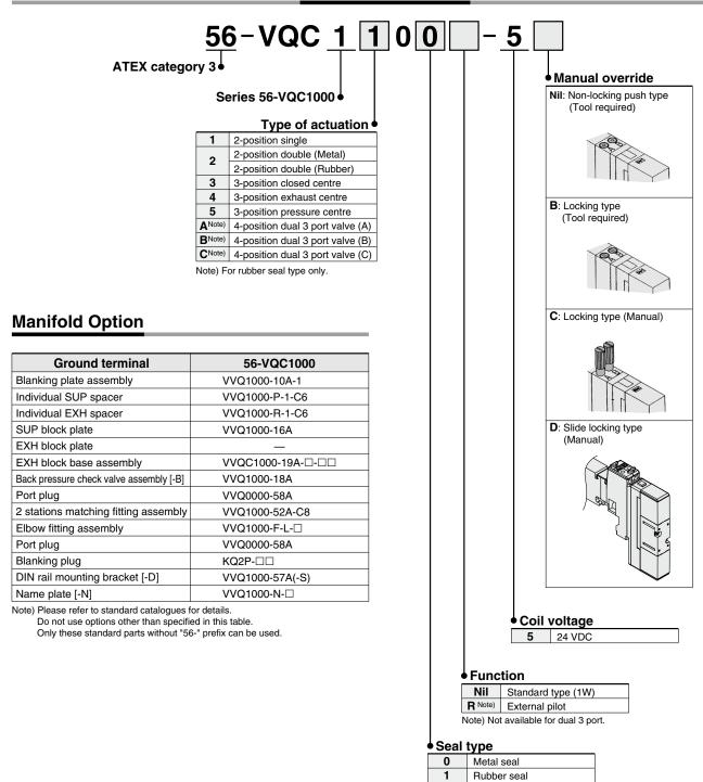
Note) "56-" solenoid valve should be installed in "56-VV5QC11" manifold. Power consumption when starting is 1W, when maintaining 0.35W. "56-VQC" solenoid valve has no polarity"
