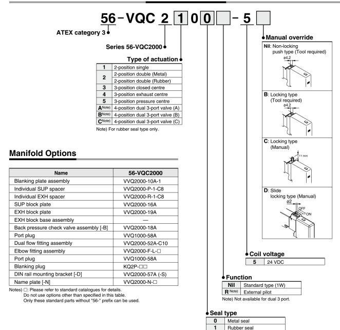
Note) "56-" solenoid valve should be installed in "56-VV5QC21" manifold. Power consumption when starting is 1 W, when maintaining 0.35 W. "56-VQC" solenoid valve has no polarity.
